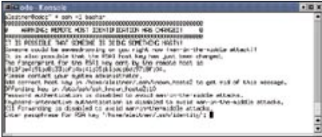
Figure 5: During the Ettercap attack (Figure 4), the client (odo in this case) receives a fake host key from the server. The key is from the attacker and not from the requested server (bashir). If the user chooses to ignore the warning, the connection can be sniffed.
